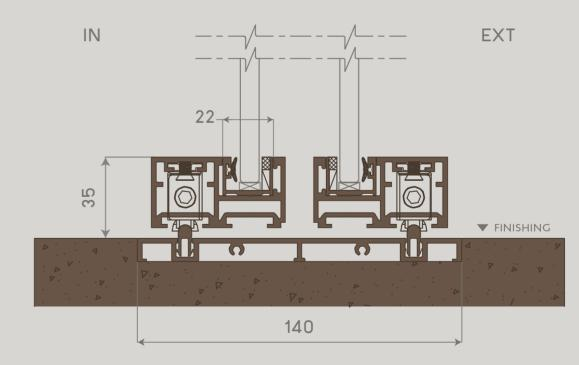
I. IO years guarantee powder coating 2. Temper , Energy , SGP glass optional 3. Flush lockable hardware 4. Backed by the AB&W warranty I year moving parts , 2 years non moving parts
